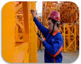
3.In order to guarantee the reliability of tower crane quality and reduce the cost, all raw materials are directly supplied by famous brands like Baosteel and Wisco. Raw materials for main parts such as standard section main limbs, tower caps adopt Q345B steel, thus the tensile strength increased by 30% and the tower crane becomes more safe and reliable.
