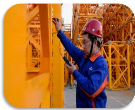
3.In order to guarantee the reliability of tower crane quality and reduce the cost, all raw materials are directly supplied by famous brands like Baosteel and Wisco. Raw materials for main parts such as standard section main limbs, tower caps adopt Q345B steel, thus the tensile strength increased by 30% and the tower crane becomes more safe and reliable.
