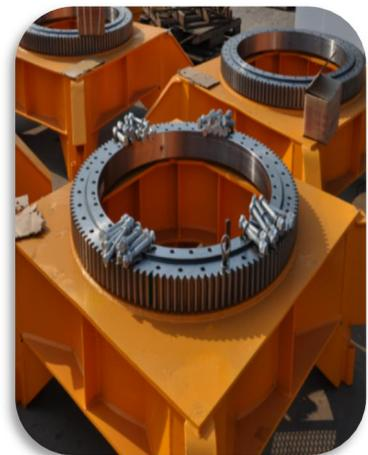
6. Attention to detail quality. High-strength bolt adopt shipborne scale DACROMET technology. It can keep not rusted for ten years .Swiss screw-thread bolts of preload promote 30 percent than traditional bolts. Weight limiter uses the tension ring structure and cast aluminum shell used Hoisting, derricking limiting stopper to extend service life.
